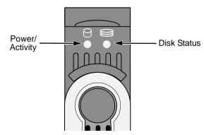
Figure 3. VTrak M500f/i/p disk carrier LEDs
